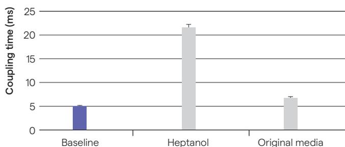
**Figure 4.** Change in signal propagation upon heptanol treatment. Cryopreserved cardiomyocytes were thawed and cultured 47 days. Treatment with 0.5 mM heptanol (reversible gap-junction inhibitor) increased coupling times between cells (i.e. between electrodes). Washout of drug restored the original untreated coupling time. Matrix analysis confirmed that the heptanol-induced increase in coupling time was observed throughout the MEA.
