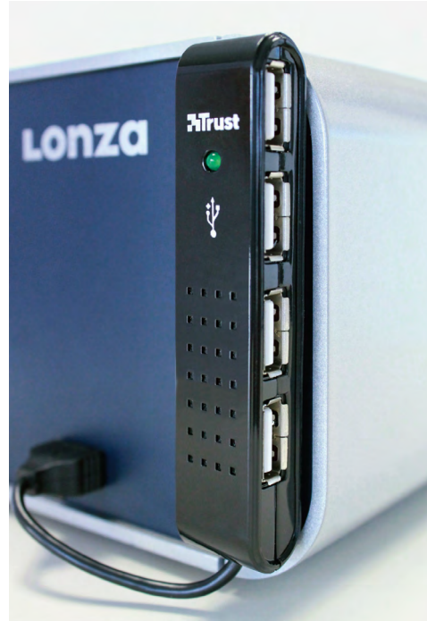
Figure 1: Recommended position for attachment of USB hub
