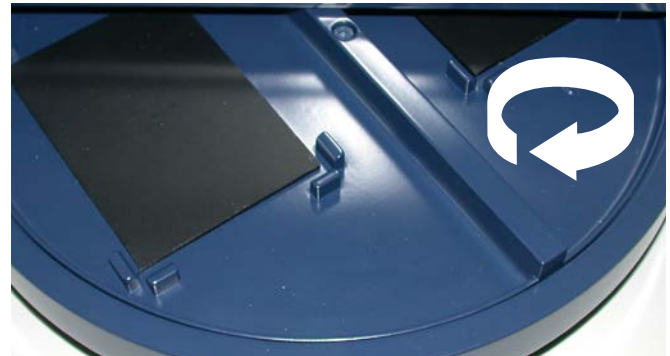
Figure 4.3: Turn carousel manually to recover samples
