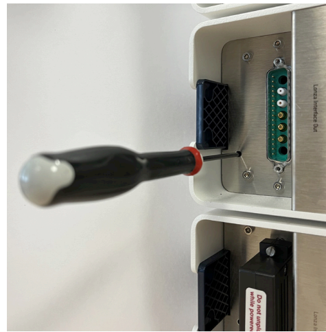
Figure 5: The position of hexagon screwdriver during manual adjustment of 4D-Nucleofector® System to the transportation mode.
