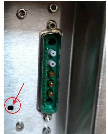
Figure 4: (A/B) Opening for hexagon screwdriver on the back of 4D-Nucleofector® System.
