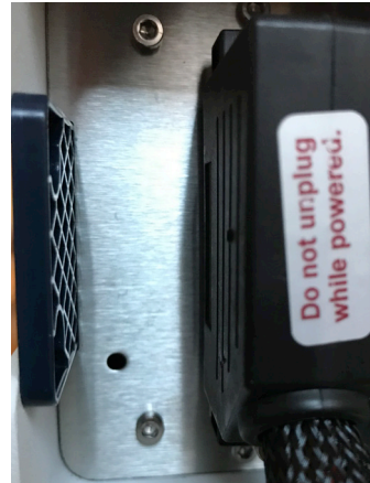
Figure 4: (A/B) Opening for hexagon screwdriver on the back of 4D-Nucleofector® System.
