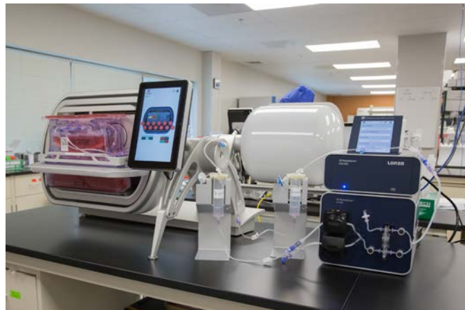
Figure 1: Cocoon® Platform integration to the 4D-Nucleofector® LV Unit via functionally-closed tubing connections. Standard Nucleofection® Process tubing set with the 4D-Nucleofector® LV Output Reservoir connected to the Cocoon® Platform
