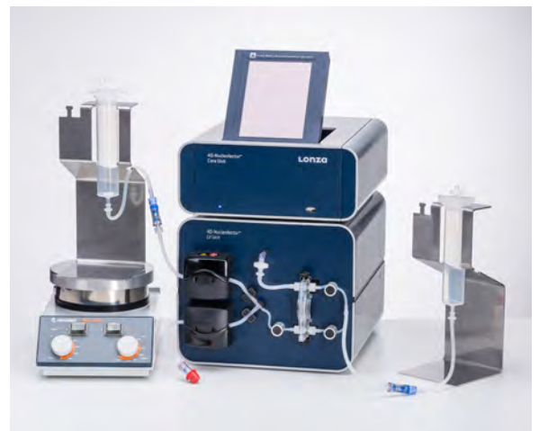
4D-Nucleofector ® System with Core and LV Unit and mounted LV Nucleocuvette ® Cartridge
