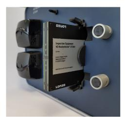
Test cartridge inserted into 4D-Nucleofector™ LV unit
