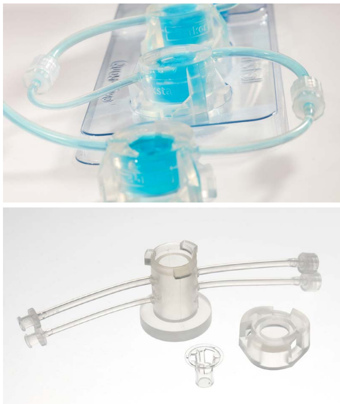
Figure 1 Quasi Vivo® Interconnected System [op], QV600 ALI [bottom] [Lonza, cat. no. QVTWSK]. Quasi Vivo® QV600 Silicone Chambers in which cell culture inserts are introduced and allowed to hang from the inner lip of the base of the chamber, the lid is fastened to seal in and immobilize the insert while culturing the respiratory epithelial cells.
