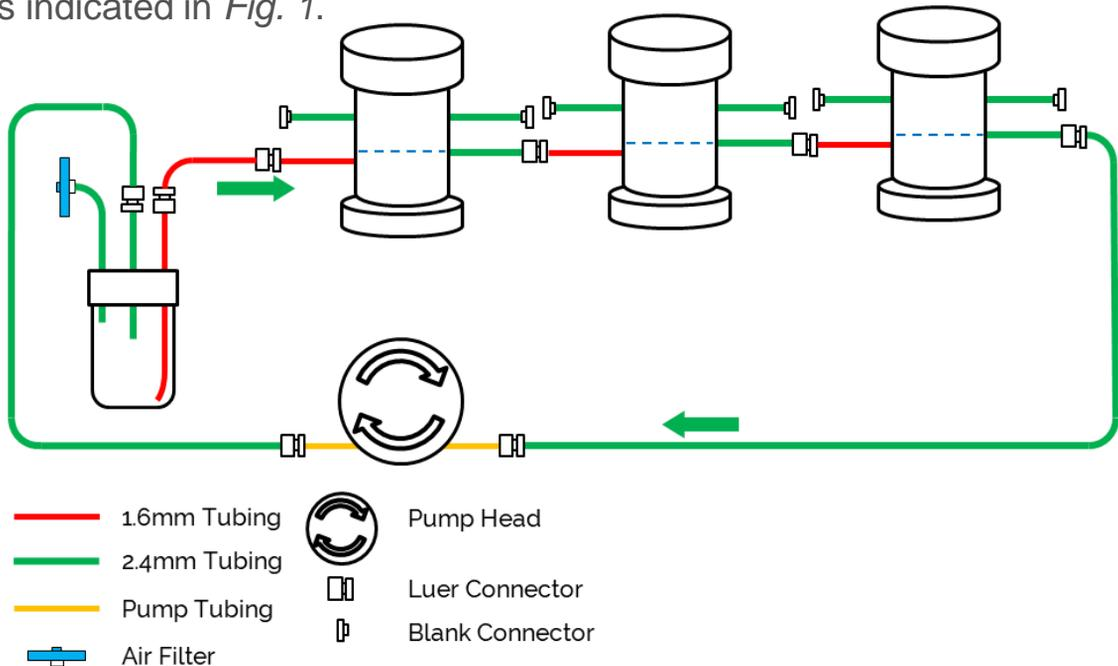
Some tubing will require the fitting of an appropriate luer lock; use the figure for guidance. Use the loading tray provided to hold the reservoir bottle and chambers in place.
