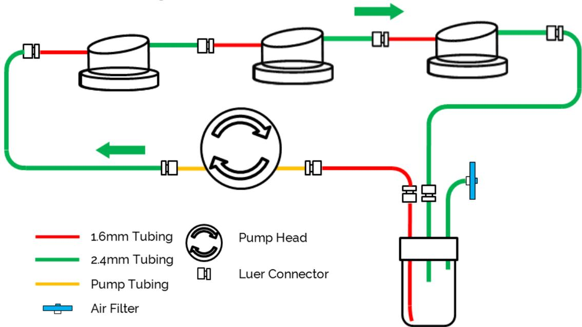
Some tubing will require the fitting of an appropriate luer lock; use the figure for guidance. Use the loading tray provided to hold the reservoir bottle and chambers in place.
