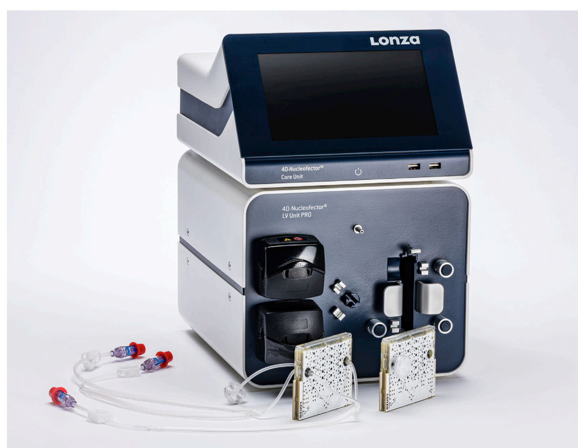
Figure 1. 4D-Nucleofector ® Core Unit with LV Unit PRO, fixed volume 2 mL Nucleocuvette ® Cartridge PRO (LV PRO FV) and flow-through LV Nucleocuvette ® Cartridge PRO (LV PRO FT). The LV PRO FV enables transfection of fixed volumes of cells, namely 0.5, 1.0, 1.5 or 2.0 mL, while for the first generation LV FV cartridge the volume is set at 1 mL. The automated LV PRO FT can process up to 20 mL T-cell suspension. Cell densities tested range from 2.5 \times 10^7 to 1.0 \times 10^8 cells/mL.
